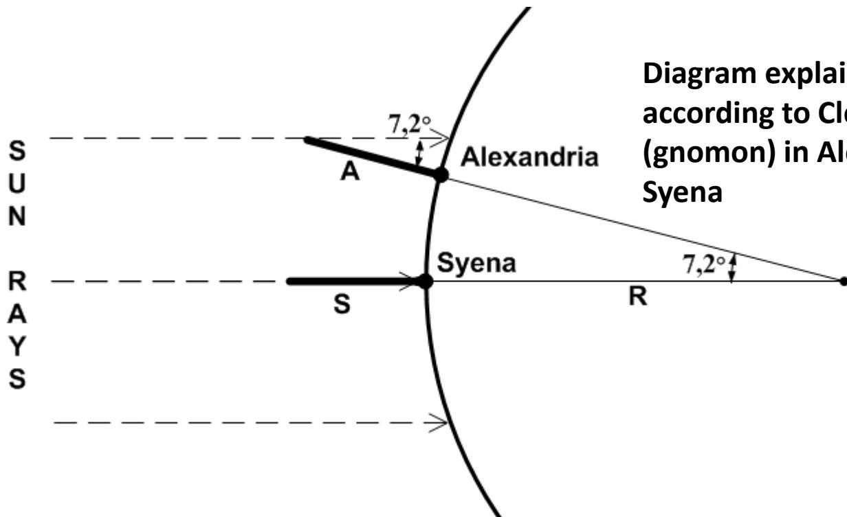
Diagram explaining the Eratosthenes' method according to Cleomedes: A - vertical rod (gnomon) in Alexandria, S - vertical rod in Syena
